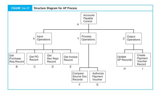
In the loosely coupled system, the process starts with Module A. This module controls all the data flowing through the system. The other modules interact only with this module to send and receive data. Module A then redirects the data to other modules.
